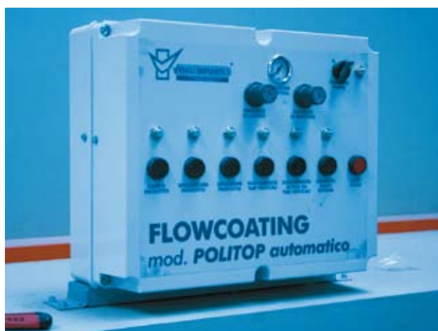
5 – Dettaglio del sistema di comando del flow-coating . 5 – Details of the flow-coating equipment command system.
